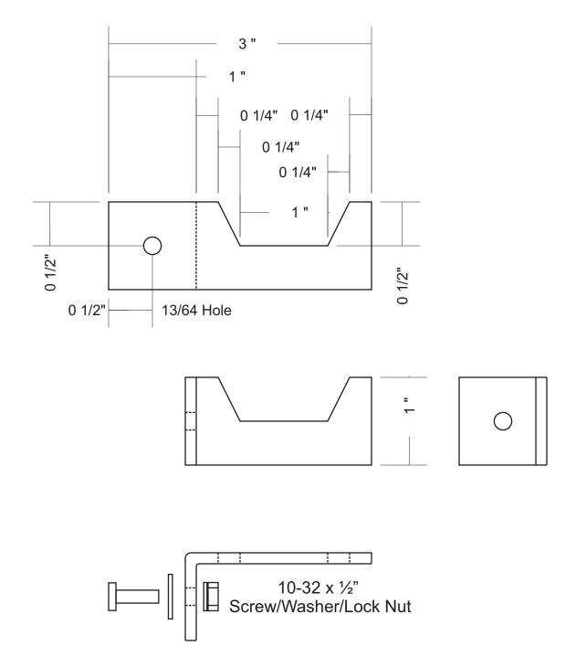
Make 3 brackets, mount them around smoker body between the existing brackets. Drilling the mounting holes 4 3/8" below the upper bracket mounting screws (or 5 1/4" below the top rim of the smoker body) will center the rack between the existing brackets.
